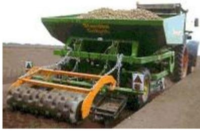
The outcome of the Standen Goliath design concept is that with the need to "refuel" much reduced, thanks to the 4 tonne tank, and the ability to drive at a much faster forward speed, the new Goliath will allow close on double the output of a conventional planter - without the need for an excessively high horsepower tractor. Its retail price will be in the range of £22,000 to £25,000, the exact price depending upon the specification selected.
